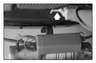
3. Turn the clip so that it is perpendicular to the pin. Pin is shown off of the vehicle for clarity.
